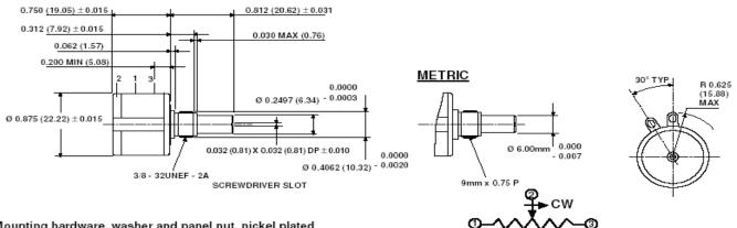
Mounting hardware, washer and panel nut, nickel plated
